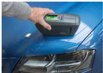
4. Take the reading two more times so you have three readings. For better colour accuracy it is advisable to move the spectrophotometer to a slightly different position with each reading. The spectrophotometer always takes three readings for unlinked readings, also with solid colours.
